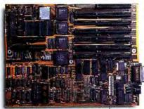
Seven industry-standard expansion slots; 1 PCcompatible slot, 6 PC ATcompatible slots, including two AST FASTslots. FASTslots provide no wait state operation with a high-speed direct interface to the 10MHz 80286 processor. Advanced architecture accommodates the next generation of accelerator and highperformance enhancement cards. It's also an open architecture for easy development and system integration
