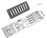
8 port, intelligent serial controller with 3% response degradation. Includes 8 MHz 80186 with built in DMA . . . . . . . . \$1299
