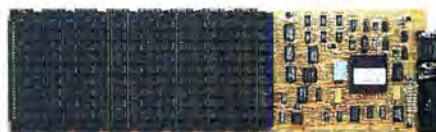
Supermax/EMS, a full 16MB of RAM for the AT and XT 286.
