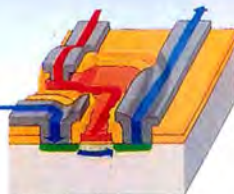
How a transistor operates as a switch.
