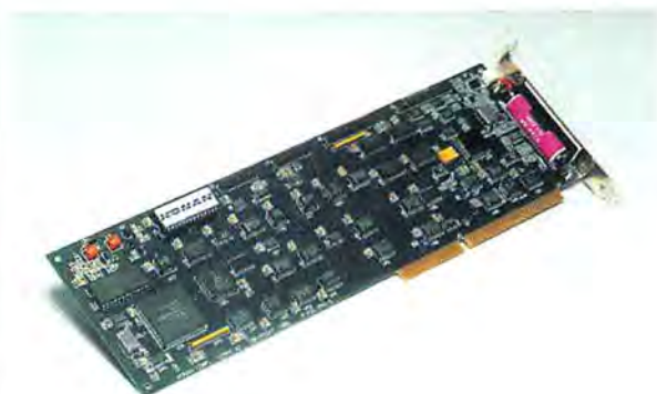
Ten Time is a 16-bit intelligent controller that employs a 1:1 interleave, zero latency, and disk caching to reduce your disk I/O to eye blinks.
