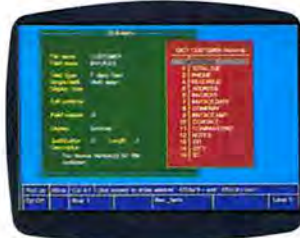
Advanced Revelation's dictionary builder allows you to specify the names, output formats, edit patterns, data conversions, formulas for your fields.
