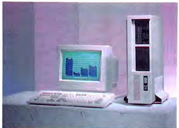
The Super-286 is an AT-compatible file server that Hyundai offers as a building block for use with a low-cost LAN.
