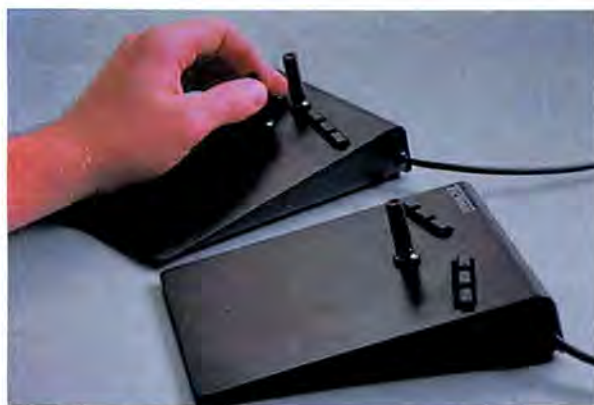
Force Stick looks like a joystick but uses force transducer technology for extreme sensitivity in high-precision CAD, CAM, or CAE applications.
