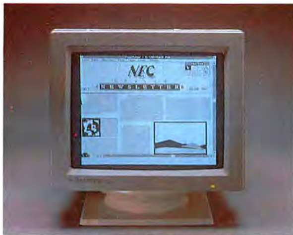
NEC's MultiSync GS offers up to 64 shades of gray in place of color images plus compatibility with graphics standards from MDA through VGA.
