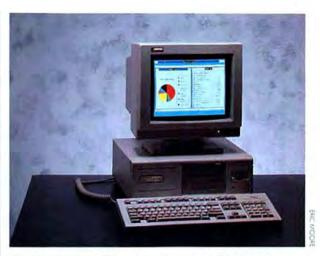
Compaq's Deskpro 386s takes advantage of Intel's new 16-MHz processor to deliver inexpensive 80386-based computing in a small package.
