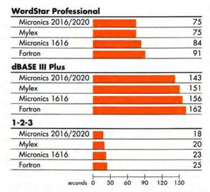
All motherboards were tested on an IBM PC AT model 339 with a 30MB hard disk and an IBM EGA board with 256K of video RAM.
