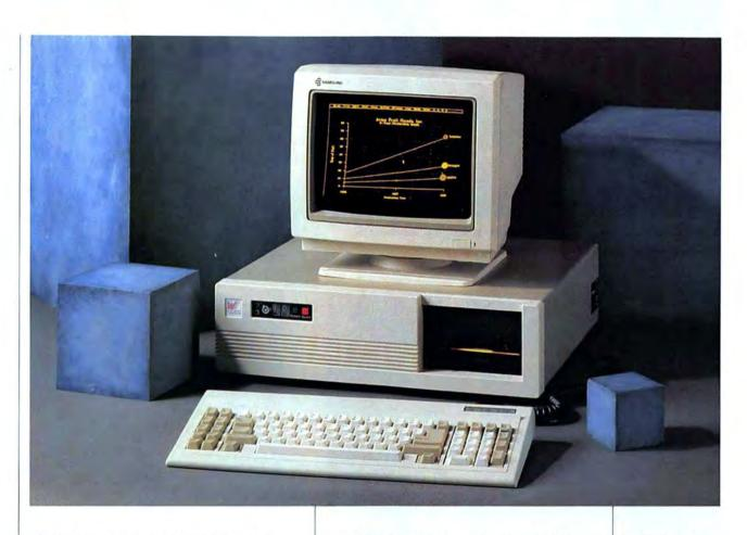
CPU switchable between 4.77 MHz and either 8 or 10 MHz, and each offers a socket for an 8087 math coprocessor. All have 135-watt power supplies and two empty half-height disk drive bays.
