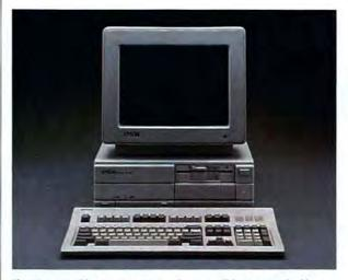
The AT-compatible Epson Equity II + has a small footprint and adds a faster 80286 microprocessor with switchable clock speeds of 8 MHz and 12 MHz.
