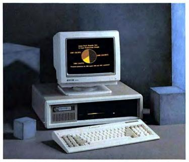
The Maxum Turbo XE runs at a maximum clock speed of 8 MHz and, unlike the other clones, allows you to install up to 1MB of RAM on the motherboard.
