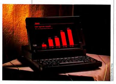
The GridCase 1520 is one of the first battery-powered 80286 laptops to reach the market—and it also offers unusually large memory expansion capacity. The combination makes it a breakthrough machine in a world of (mostly) 640K, 8088-based battery laptops. Unfortunately, its brief 45-minute battery life and long case (15 by 12 inches) make it less than ideally suited for airplane computing or operations away from a wall plug.
