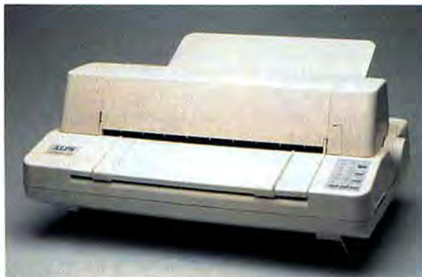
The flatter the better is the motto of the ALPS Allegro 24, a 24-pin dot matrix printer that reduces jamming by feeding paper directly over a flat, stationary platen and under a downward-striking printhead. It prints 180 cps in draft mode and 60 cps in letter quality mode.
