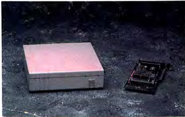
NetLine's LINK solves the LAN cable jumble by using the electrical wiring already in your walls as a transmission medium. The token-passing bus network has a 2000-foot range and moves data at 19,200 bits per second.
