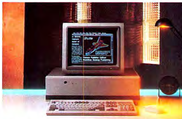
ALR's desktop version of its 80386 tower offers the same CPU and proprietary cache scheme featuring 64K of 25ns static-column RAM.
