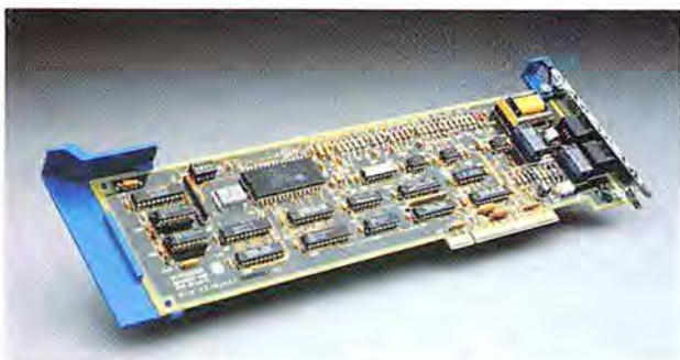
JT Fax PS/Q turns a PS/2 or compatible into a group III fax machine with a 4800-bps chip that converts and sends in a single step.
