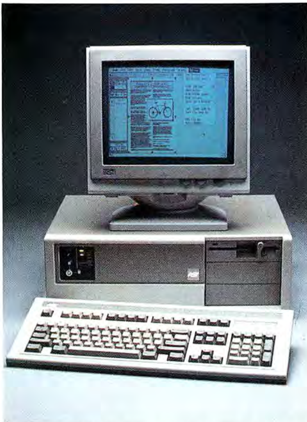
The Premium/286 Model 140V comes standard with VGA graphics, a 10-MHz 80286 processor, a 40MB hard disk, and seven expansion slots.
