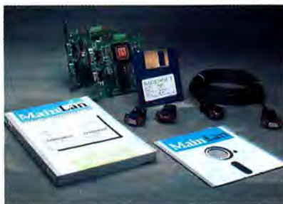
The MainLan Starter Pack—everything you need to connect two computers, including two network boards, software, documentation, and one 16.5' shielded cable with terminating plugs. The Extension Pack contains the network board, and one cable and plug set.
