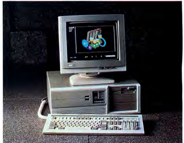
Each of AST's new cast of 80386-based computers includes at least 32K of zero-wait-state memory caching that enhances performance by as much as 30 percent.
