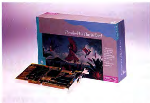
The Paradise VGA Plus 16 offers 16 colors from a palette of 262,144 at 800 by 600 resolution as well as the blazing speed of a 16-bit data path and a 16-bit video BIOS.
