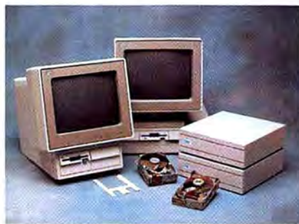
IBM® PS/2 Models 25, 30 and 30-286 Solutions: (Internal) 20, 30 and 40 MB; 40-24 ms. (External) PC Stack: 30, 45 and 80 MB; 40-28 ms.
