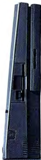
T3200: 12MHz 286, 2 IBM compatible slots, 40MB hard disk, 1.44MB floppy, 1MB RAM expands to 4MB, EGA screen.
