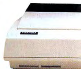
P351SX: 360/120 cps, 24-pin letter quality, color option, Toshiba/Quume and IBM emulations standard, Epson & Diablo emulations optional.
