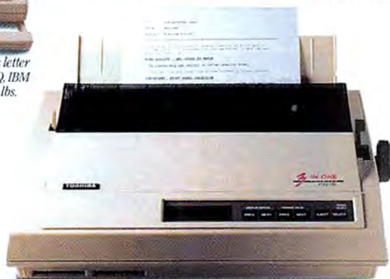
P321SL/SLC (color): 216/72 cps, 24-pin letter quality, up to 360x360 DPI graphics, Toshiba/Quine and IBM emulations standard, Epson and Diablo emulations optional, 32KB print buffer, front panel controls, advanced paper handling.
