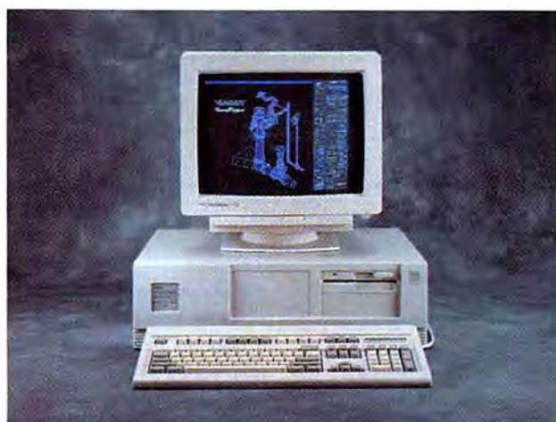
NEC's PowerMate 486/25E includes a bus-master hard disk controller, a secondary cache for the 486, and accommodations for up to 64MB of CPU-speed RAM.
