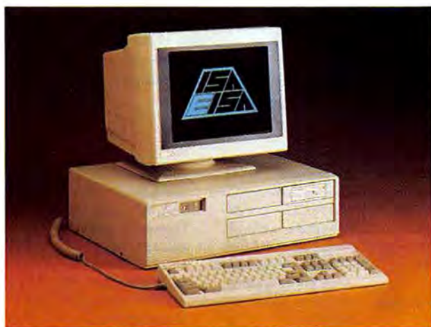
The Zenith Z-386/33E couples an EISA bus with an intelligent controller that can handle four ESDI, seven SCSI, and two floppy drives.
