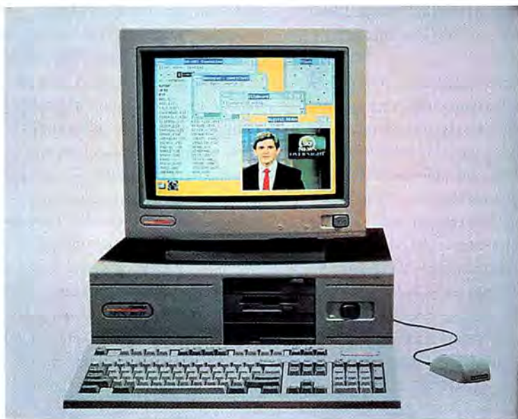
VideoLogic's Digital Video Architecture products let you display and manipulate full-motion video on a standard VGA monitor. One option uses Windows or OS/2 to run video alongside other applications.
