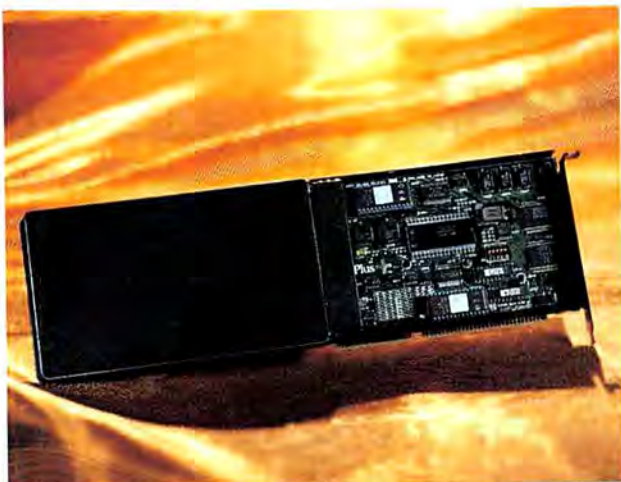
The Hardcard grows up, adding a 16-bit interface and easy installation for DOS, OS/2, or PC LANs.
