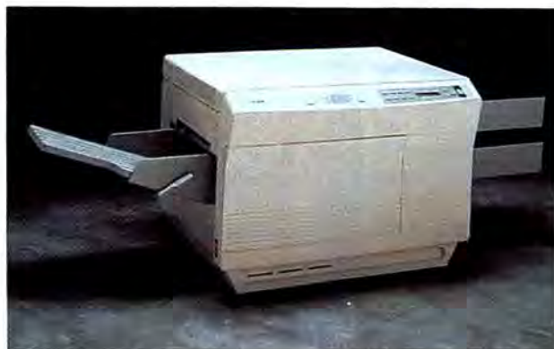
Built around an LED rather than a laser, the LPX 2020 printer achieves high throughput for both text and graphics by coupling ALPS's own 20-ppm engine with a controller powered by National Semiconductor's 15-MIPS 32GX32 processor and backed by up to 8MB of memory.
