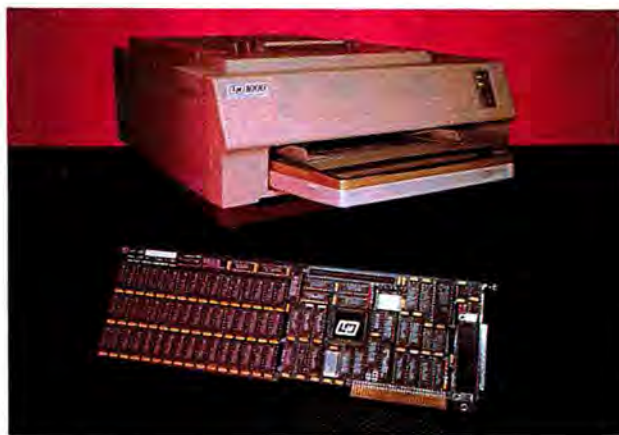
The LaserMaster 1000 Plain-Paper Typesetter brings you typesetter-quality, 1000-by-1000-dpi resolution in a box not much larger than a Hewlett-Packard LaserJet Series II, thanks to a special TurboRes controller card with a proprietary processor and 6MB of memory.
