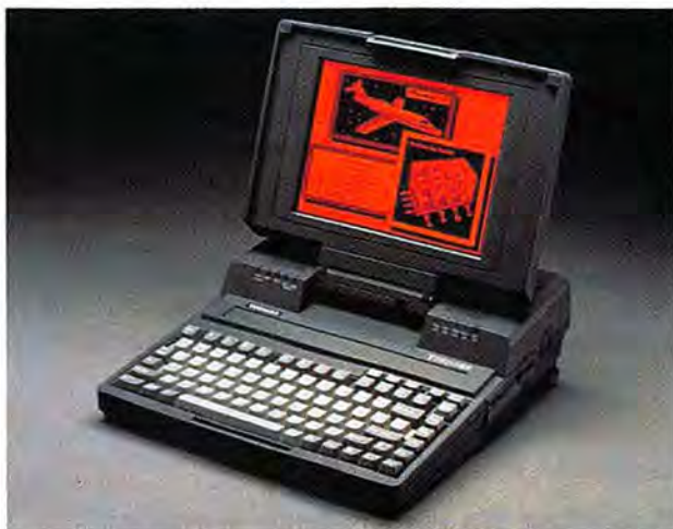
Toshiba's new T3100SX is a battery-powered version of its T3100e, with an even brighter VGA gas plasma display that shines for 3½ hours on two rechargeable nickel-cadmium batteries at 640 by 400 resolution.
