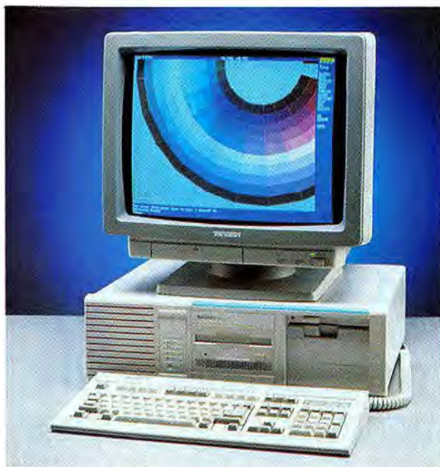
The Tandon 486/25 beefs up the power of the i486 processor with a 64K memory cache on the motherboard and a fast EISA bus.
