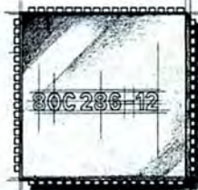
A 12/6MHz 286 microprocessor makes the T1200XE one of the most powerful notebooks available.
