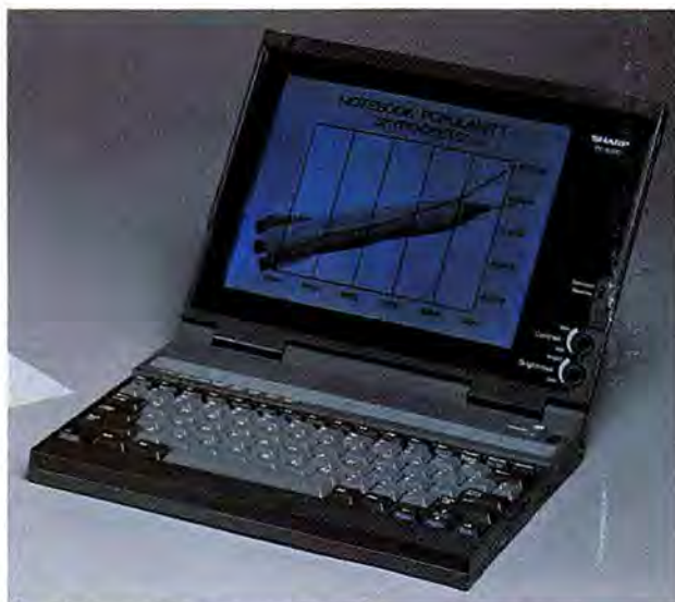
Sharp's new PC-6220 is a superlight notebook PC with VGA graphics, 286 processor power, and a fast 20MB hard disk.
