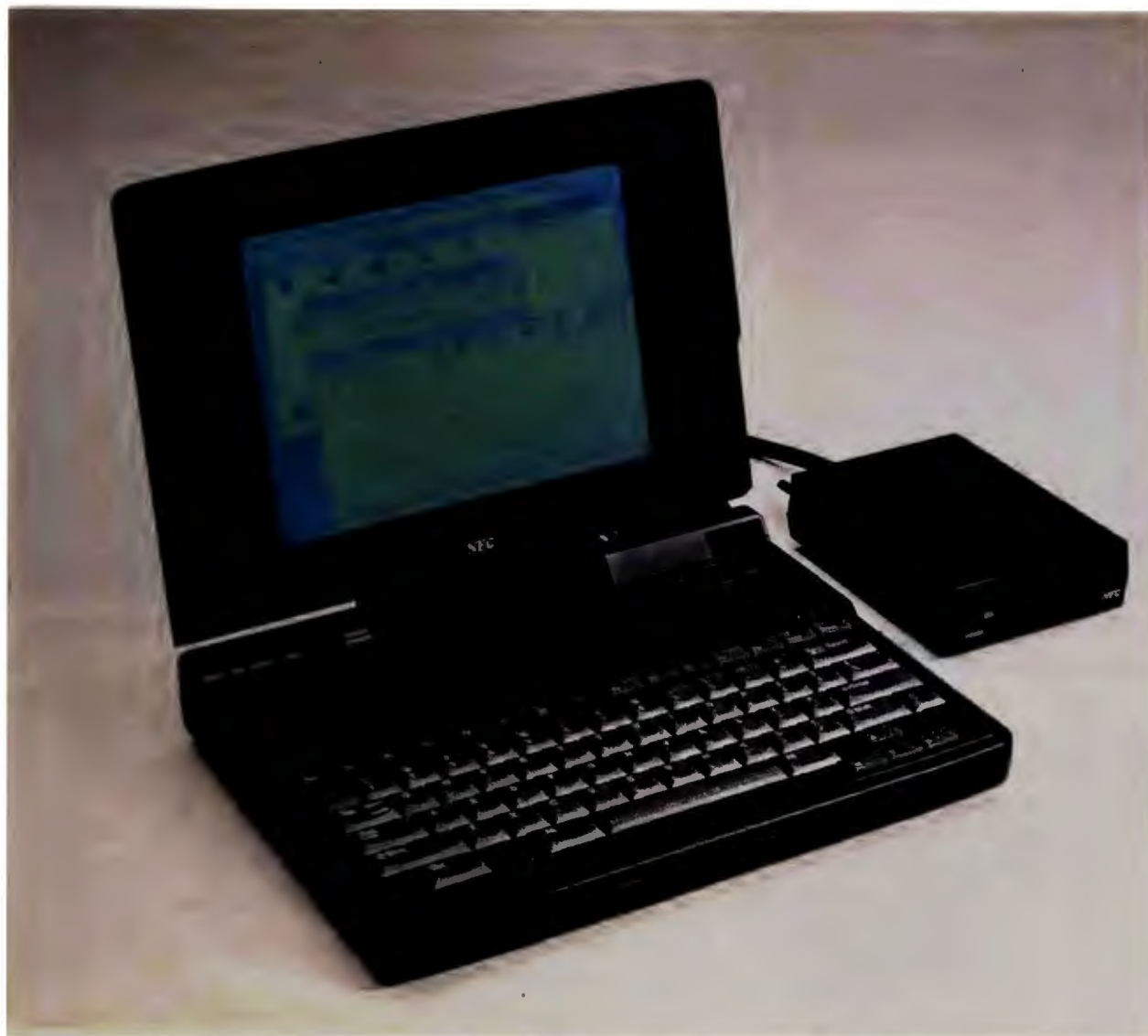
With a VGA display, a 20MB hard disk, and a 12-MHz 286 CPU, NEC's UltraLite 286V is more usable than the original, driveless UltraLite.
