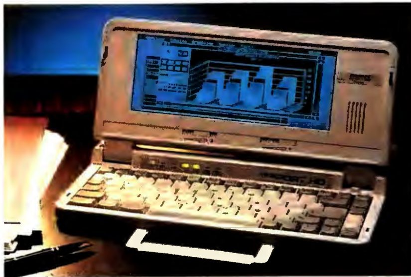
Zenith's 15-month-old MinisPort notebook makes a good move with a 23ms 20MB hard drive and an external 3½-inch floppy drive.
