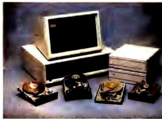
Compaq® Deskpro Series Solutions: (INTERNAL) 20, 40, 60 and 80 MB; 65-28 ms. (EXTERNAL) PC Stack: 45 and 80 MB; 40-28 ms.
