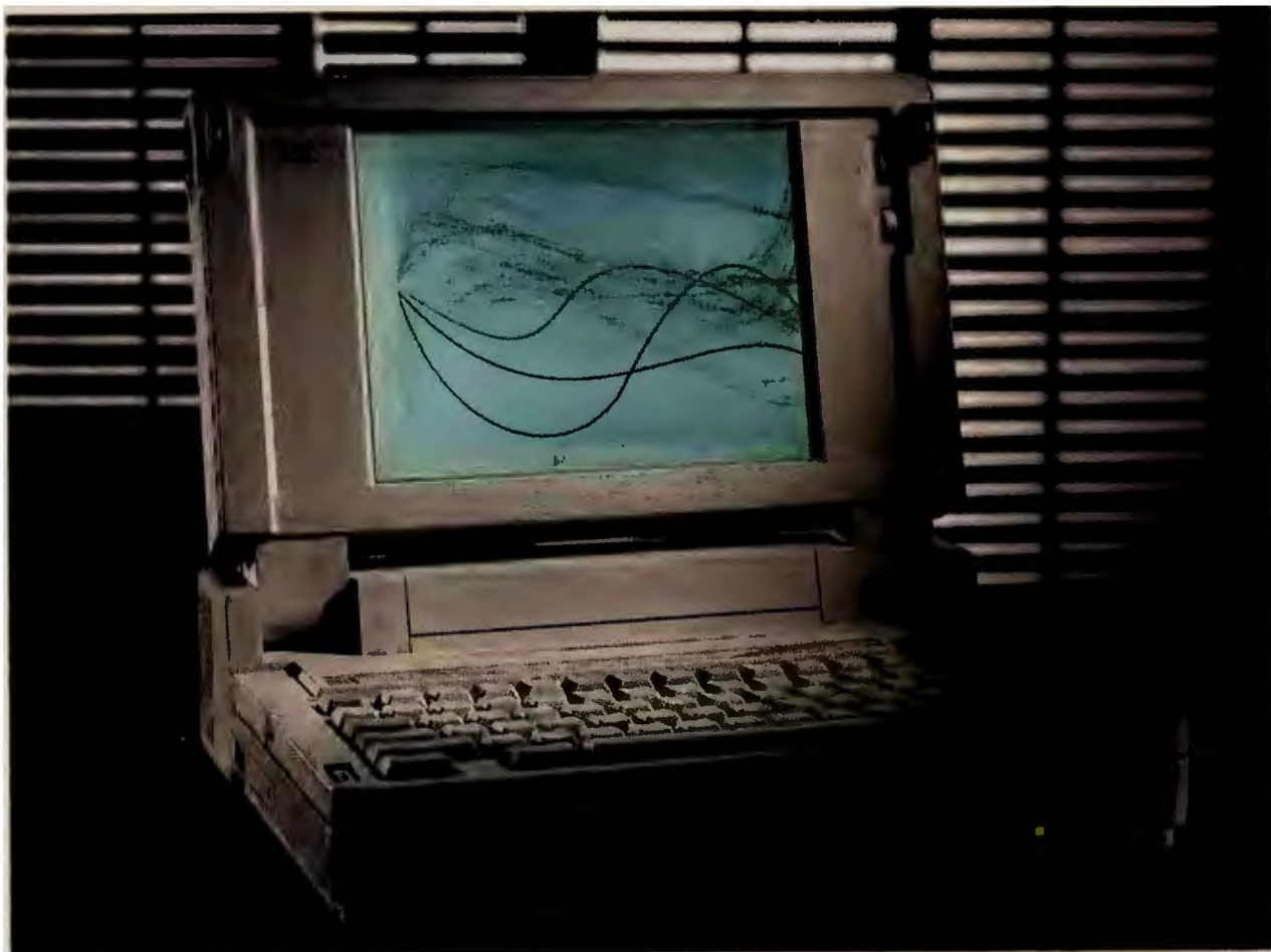
NEC's ProSpeed SX/20 offers desktop performance in a 12½-pound package, with a VGA screen, a 20-MHz SX CPU, and an 80MB hard disk option.
