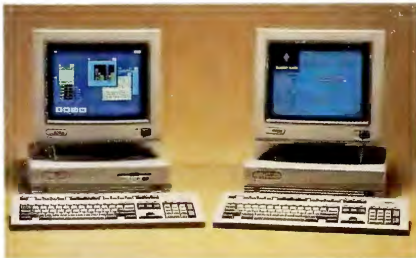
Compaq's Deskpro 386N (left) and 286N (right) diskless workstations offer data security and ROM-based configuration and diagnostics.
