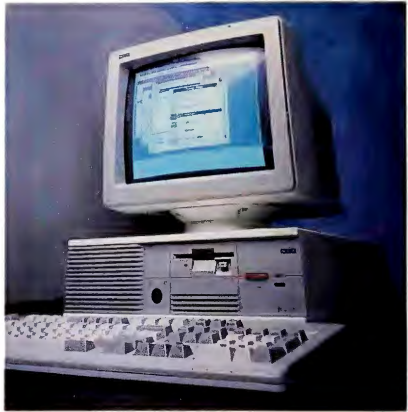
NCR's PC486/MC33 is a 486-based system that takes advantage of Micro Channel architecture, custom ASICs, and plenty of memory for maximum throughput during multiple operations.
