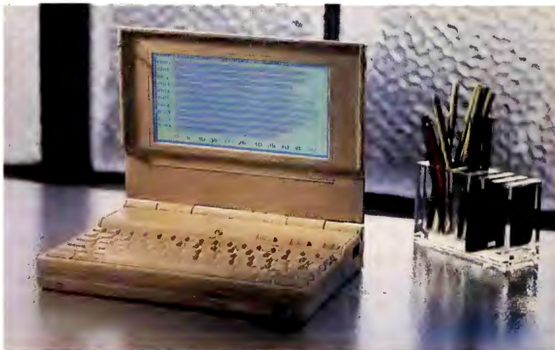
Compaq's LTE is the fastest 8086-based notebook we tested, and it boasts an outstanding battery life of 5 hours in normal use. Unfortunately, it's relatively heavy.
