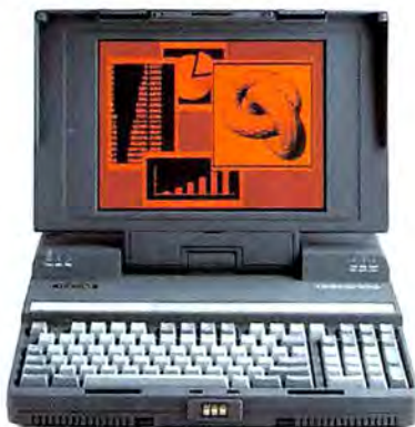
T5200. 386 microprocessor, 40, 100 or 200MB HDD, 2 to 14MB RAM, 2 IBM-compatible expansion slots (in addition to dedicated memory slots), VGA plasma display.
