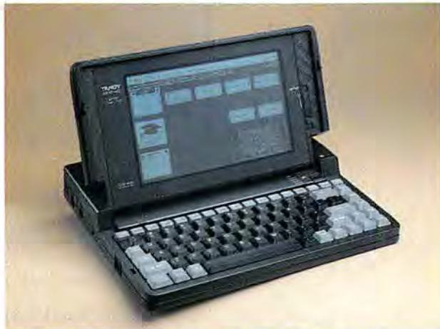
The Tandy 2810 HD typifies new standards in 286-based notebook portables: VGA display, on-board floppy, and 20MB hard drive.
