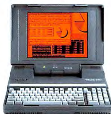
T3200SX. 386SX microprocessor, 40 or 120MB HDD, 1 to 13MB RAM, 2 IBM-compatible expansion slots (in addition to dedicated modem and memory slots), VGA plasma display.
