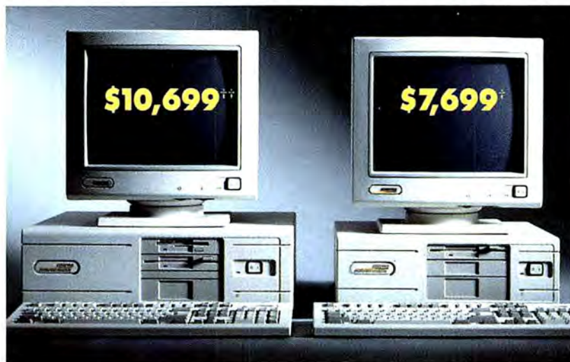
Compaq's 33 MHz and 25 MHz 386 computers. System includes: VGA Color monitor, 120 MB hard drive, 4 MB RAM.
