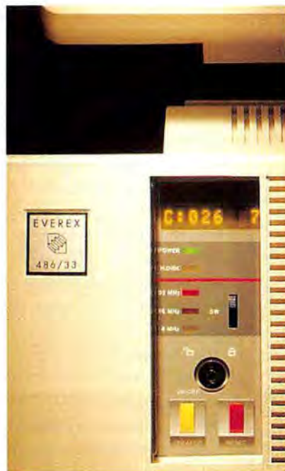
The fast, relatively inexpensive Everex Step 486/33 sports a front panel with a reset button, an LED diagnostic display, a speaker on/off switch, and a speed switch.
