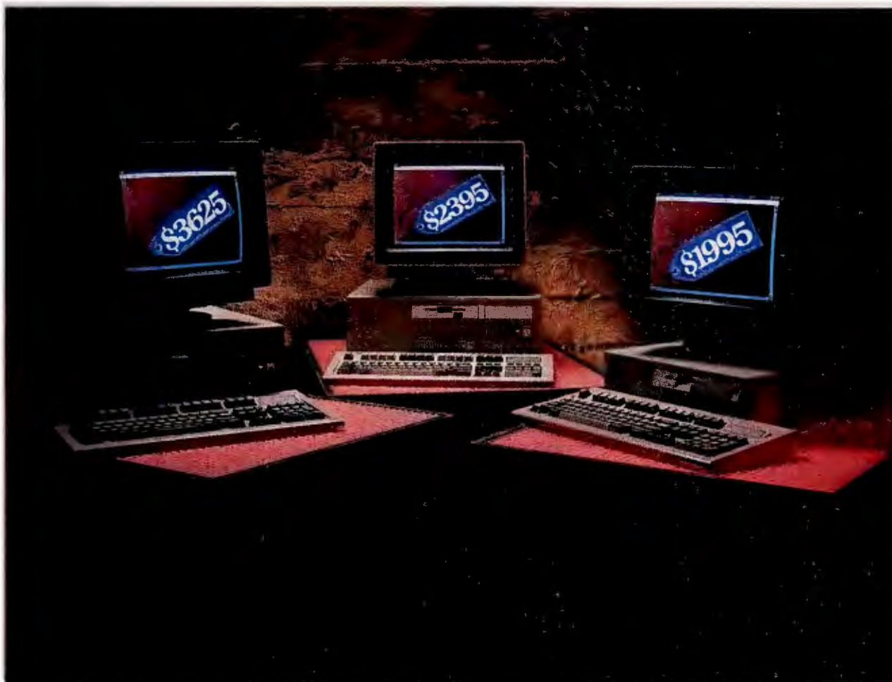
PS/2 Models 57, 40, and 35, with base prices proudly displayed. The 40 and 35 have standard AT slots; the 57, a Micro Channel unit, comes with a 2.88MB floppy drive.
