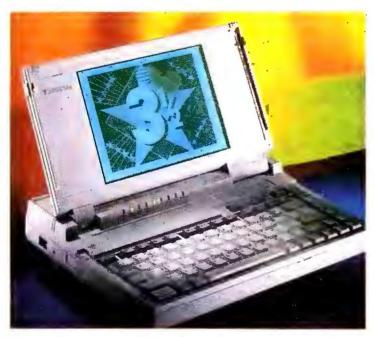
The big Toshiba gets good marks for its long-lasting and environmentally safe nickel-hydride batteries.
