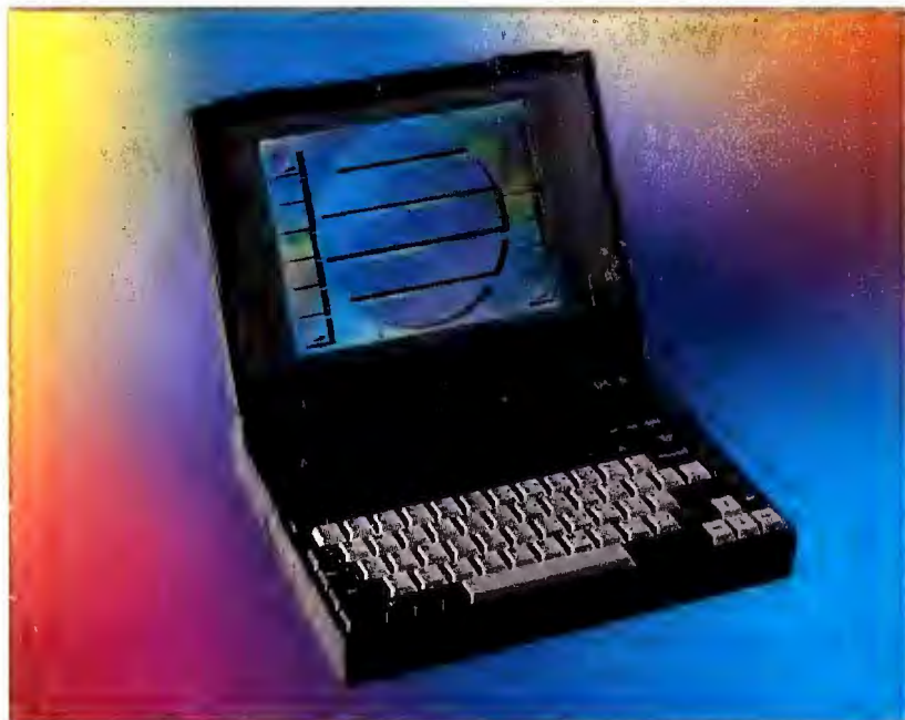
Dell's passive-color notebook, the 325NC, weighs a mere 7.1 pounds. In informal battery tests, it ran almost 3 hours.
