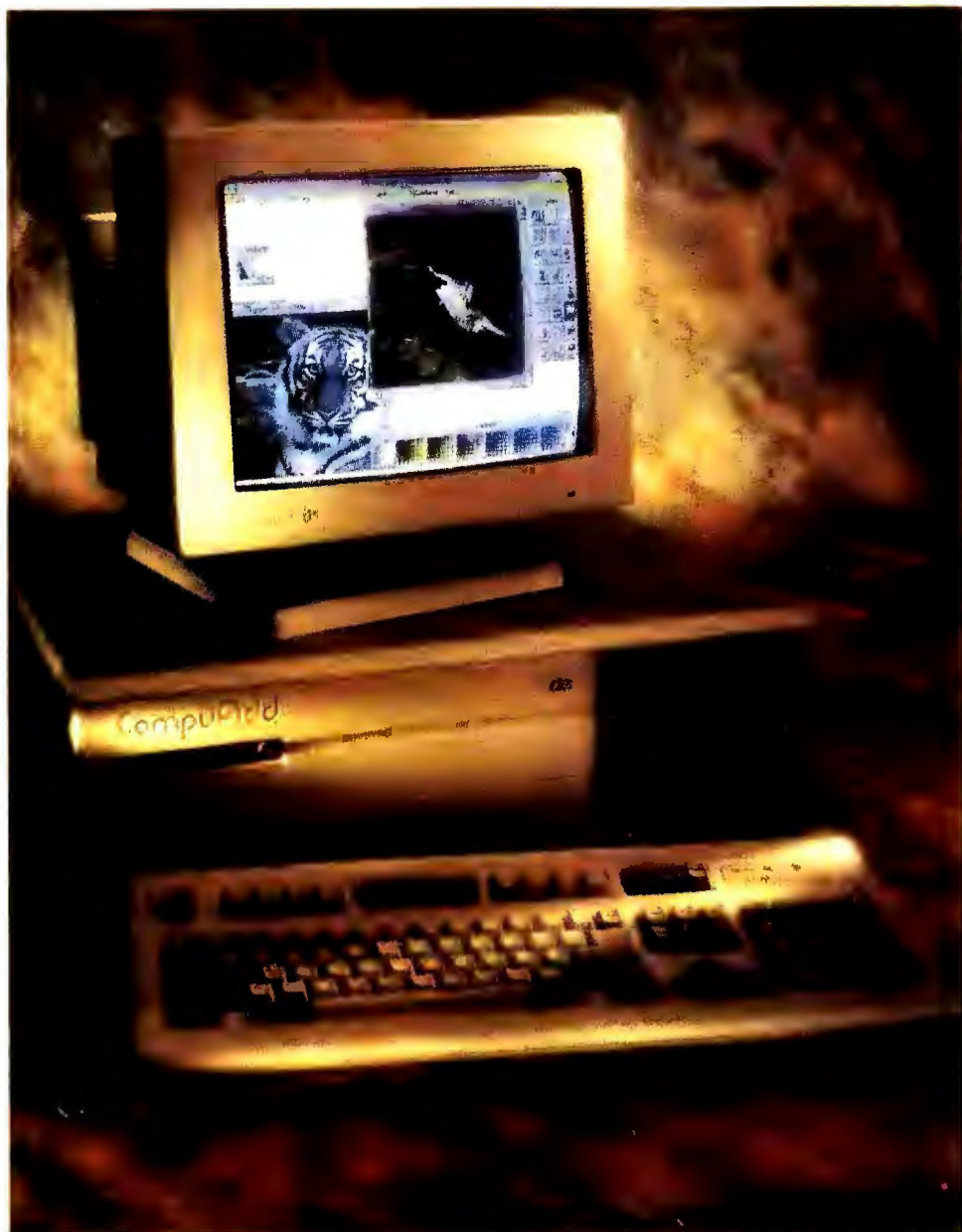
Promising faster graphics at competitive prices, CompuAdd Computer's new upgradable 486SX 420s (shown above) and 486DX 433 feature a special 12.5-MHz ISA bus slot for the company's Hi-Rez VGA video controller.
