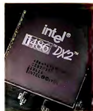
Inside, this speed demon runs at 50 MHz. Outside, it plugs into a low-cost 25-MHz memory subsystem.
