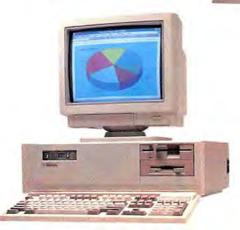
Step up to even greater expansion capability! Northgate's full-size desktop case is your best choice when space is no object. A 200 watt power supply provides plenty of power for your toughest applications. Expansion capacities include eight expansion slots plus space for three exposed and two internal 5.25" half-height devices.
