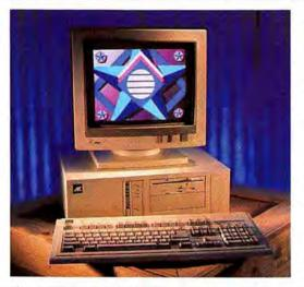
The upgradable EISA AMKLY has a removable platform for its power supply and four drive bays.
