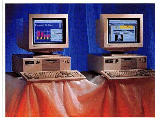
Two new color monitors match the capabilities of the video adapter. The 14-inch and 17-inch AST Super VGA-LR monitors are low-radiation displays that support resolutions up to 1024 by 768 in noninterlaced mode at a frequency of 72 Hz or 1280 by 1024 in interlaced mode at 87 Hz. Noninterlaced mode minimizes screen flicker and thus puts less strain on the eyes.
