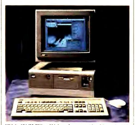
With its 486/33 CPU and high-performance video drivers, the AST Bravo 4/33 has enough horsepower to run as a network server or as a stand-alone graphics workstation.
