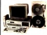
Now you can exchange data files between your IBM PC/XT/AT and any mainframe or minicomputer using IBM compatible 1600 or 6250 BPI 9-Track tape. Unit can also be used for disk backup. Transfer rate is up to 4 megabytes per minute on PCs and compatibles. Subsystems include 7" or 10½" streaming tape drive, tape coupler card, cables and software.
