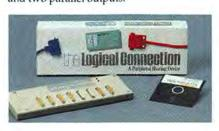
All six ports of the Logical Connection Plus are automatically configured as parallel or serial, and input or output. Versatility and high speed are key features.
