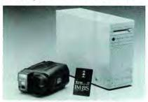
The DS-100 Memory Card Camera stores up to 21 high-resolution color digital images on each reusable Image Memory Card. The DP-100 Processor reads the cards and transfers the digital pictures directly into the PC. The camera features automatic flash and focus and a 3x power zoom lens.
