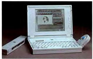
Zenith's Z-Note 386SL notebooks have built-in Ethernet circuitry and preinstalled shell software for networking.
