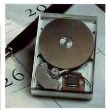
Tiny drive: HP's 1.3-inch Kittyhawk is smaller than a matchbox, stores 20MB of data.
