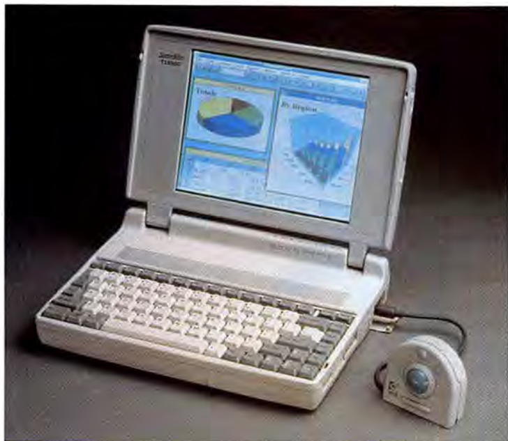
Toshiba's T1850C is one of three budget-minded portables. Its 25-MHz 386SX CPU, 80MB hard drive, 4MB of RAM, and active-matrix color cost about $3300.
