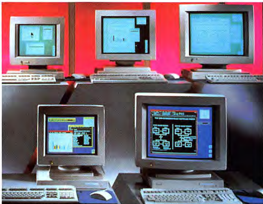
The VXT 2000 terminal family includes monochrome, gray-scale or color versions in 15-, 17- or 19-inch monitors. All VXT systems are expandable to 16 MBytes. The monitors' resolution is 100 dots/inch, with a flicker-free refresh rate of 72 hz.
