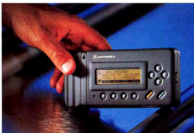
Motorola's 1-pound InfoTAC wireless radio modem operates as either a two-way messaging device or as a radio modem.
