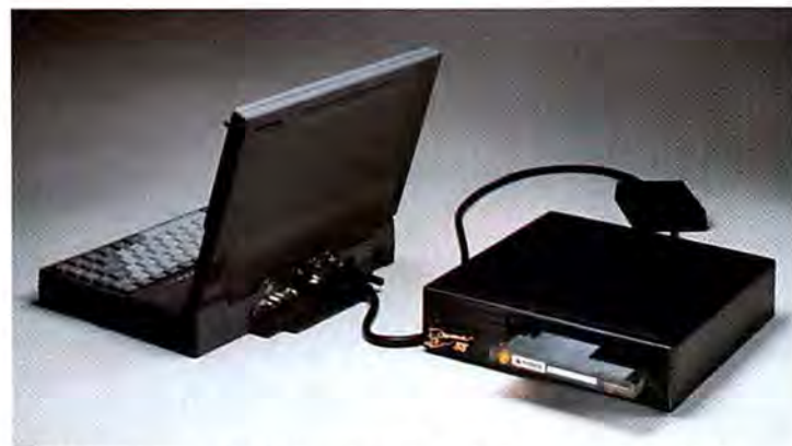
Available in 44MB and 88MB versions, the 5-inch Puma portable drive's parallel port interface makes it compatible with just about any PC or notebook.
