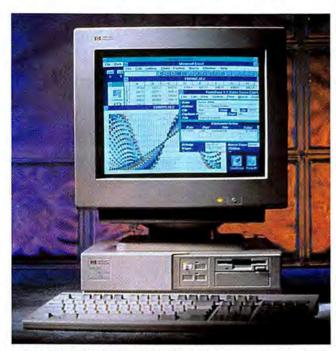
HEWLETT-PACKARD'S NEW CPU-UPGRADABLE VECTRA 486N features a proprietary local bus for faster graphics action.
