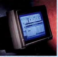
THE KANTEK ERGOVISION2 mesh filter's front-mounting design can attach to the face of the monitor or on top. The grounding wire provides antistatic protection.
