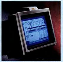
THE I-PROTECT FB mesh filter attaches to the top of your monitor. A giant Velcro strip holds the filter in place, so it doesn't crash onto your desk when it gets bumped.
