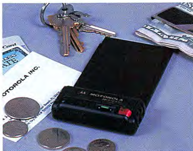
THE NEWSCARD IS THE PCMCIA VERSION of Motorola's NewsStream receiver, a one-way paging device that lets you receive E-mail, computer files, and other data while on the road.
