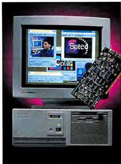
VIDEO FOR THE REST OF US: The SuperMac Technology $499 VideoSpigot is a PC add-in card that captures video.
