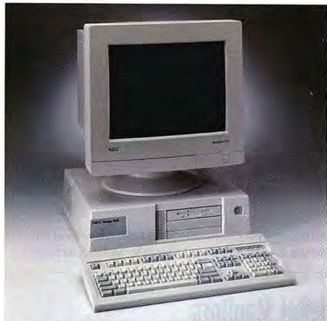
NEC'S NEW IMAGE PC, available in three 486 models, offers local bus graphics, improved hard drive performance, and a ZIF socket.
