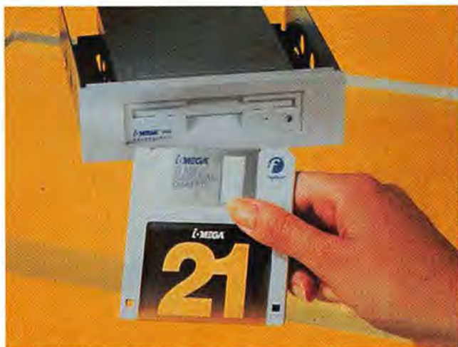
IOMEGA'S FLOPTICAL DRIVE uses 3½-inch disks that hold up to 21MB of data, yet it reads and writes to conventional floppies as well.
