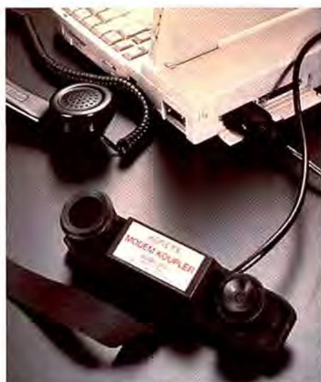
THE KONEXX KOUPLER Model 305 comes with a built-in fax-modem. You strap the coupler to the phone handset and plug the coupler cable into your laptop's serial port.
