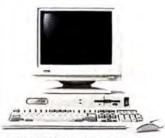
COMPAQ ProLinea 4/50 50-MHz 486DX2, 4-MB RAM, 240-MB hard drive. SVGA Color Monitor.
