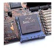
Note the extra row of pin holes. That's for the upgrade to Intel's OverDrive™ based on the Pentium™ architecture!
