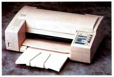
EPSON'S STYLUS 800 ink jet printer delivers 360-dpl resolution at speeds of up to 3 pages per minute. It comes with a 100-sheet paper tray and seven internal fonts (four scalable) and operates at a quiet 45 to 47 decibels.
