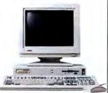
COMPAQ ProLinea 4/33 33-MHz 486DX, 4-MB RAM, 120-MB hard drive. SVGA Color Monitor.
