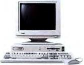
COMPAQ ProLinea 4/50 50-MHz 486DX2, 4-MB RAM. 240-MB hard drive, SVGA Color Monitor.
