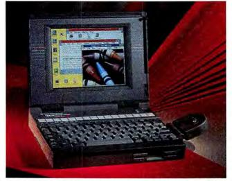
COLORFUL BUT EXPENSIVE, the \$4999 TravelMate 4000E WinDX2/50 from Texas Instruments features an 8.4-inch active-matrix color display and a proprietary local bus for fast video performance.
