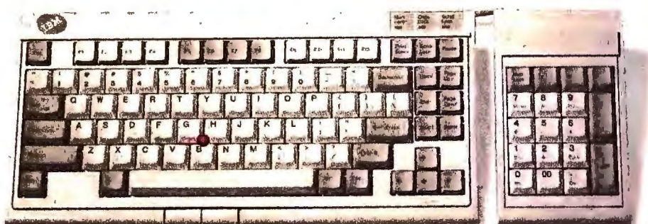
Quiet Touch Keyboard with TrackPoint II (Shown with optional numeric keypad)
