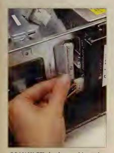
CONNECT the data cable to the new hard drive.
