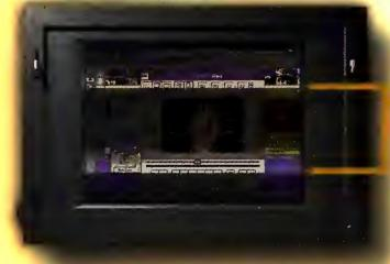
Essentially, dual-scan screens work the same as single-scan ones, except the screen is split into top and bottom halves, each with its own multiplexer. Since each area has half as many rows to cycle through as a single-scan screen, the refresh cycle is twice as fast, and image quality is better.
