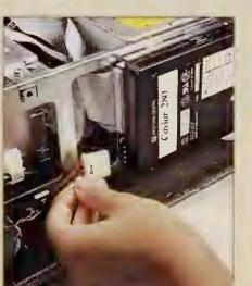
PLUG the power connector into the new drive's power socket.
