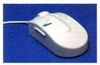
ROLLING, ROLLING: ProAgio's roller button lets you scroll through text in a window without having to click inside the scroll bars.
