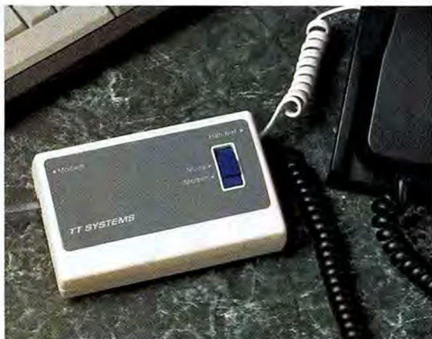
CHAT LINE: The Modem Mate MPA-100 plugs into the handset of a phone for easy modem setup on the road or in your home.
