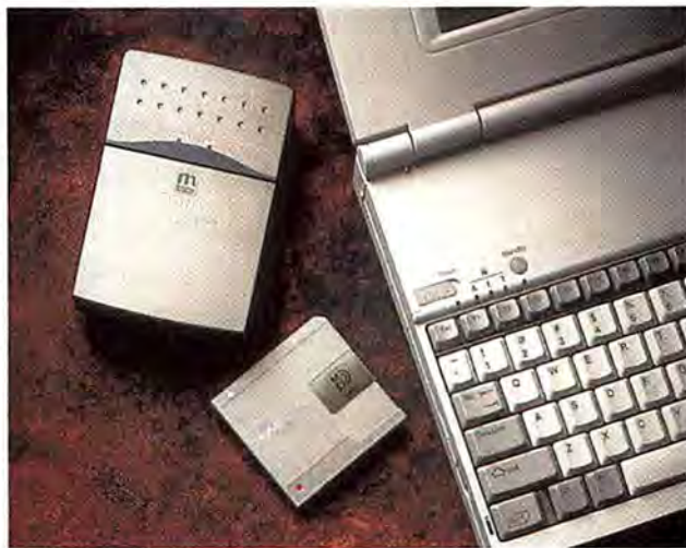
DATA TO GO: Sony's MDH-10 drive is a little bigger than a Walkman but can store 140MB of data on a 2.5-inch disc.
