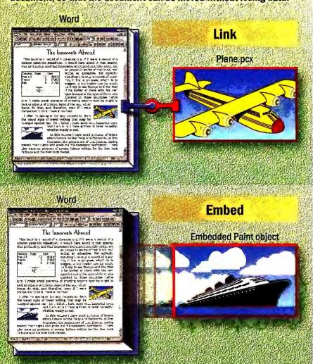
Turning a linked file into an embedded object. In the container application's Links dialog box (reached via Edit • Links in most programs), you'll find a button with the promising name Break Link. Don't touch it! If you do, OLE will convert the link into a mere picture of what was there before, not into an embedded object. This may be fine if the link was to a
