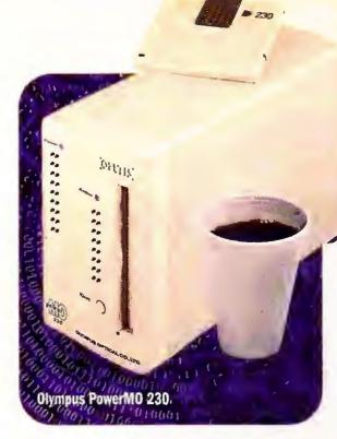
near hard disk speeds in all but the data transfer test, testimony to what a 1MB buffer and 4500 rpm can do. Such performance makes this SCSI drive a good choice for running programs or as a fine archiving device, thanks to long-lived MO cartridges.
