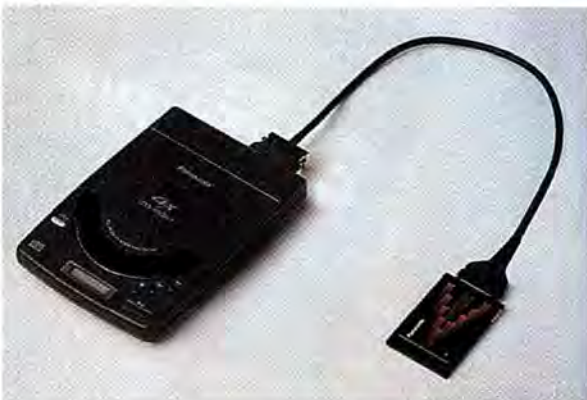
PORTABLE CD-ROM: Panasonic's KXL-D740 4X drive weighs only 14 ounces and connects to notebooks via a PC Card Type II slot.
