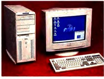
CHASSIS FULL OF CHOICES: Dell's redesigned chassis has better on/off button placement and extra drive bays.
