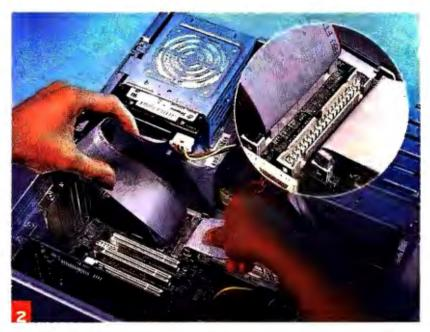
Check your connections. If your PC is less than two years old, the motherboard probably has two 40-pin EIDE connectors, with one plugged into the hard drive's cable. Don't use that cable for the CD-ROM drive. Use the cable that came with your CD-ROM drive (or buy a cable) and the free EIDE connector. PCs without EIDE connectors need an EIDE card (about \$25 if not bundled with the drive).
