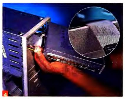
Mount the drive and install the software. Find pin 1 on the EIDE connector. The data cable's red wire (inset) must connect to pin 1. Mount the drive. Connect the data cable, then the 4-wire power cable. If you have a sound card, connect the audio cable to the drive. Install the software that came with the drive, reboot, and put the cover on.
