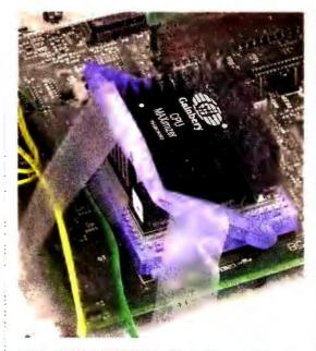
LOW-TECH SOLUTION: The only way we could fit the Gainbery upgrade chip into the IBM motherboard was with Scotch tape.
