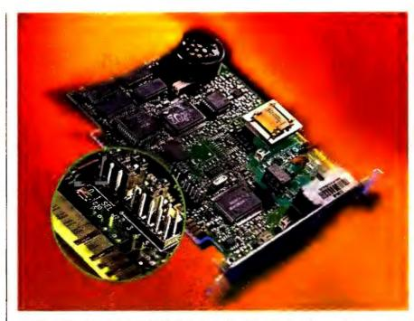
PLUG AND PLAY? MANUAL? U.S. Robotics' Sportster Faxmodem can swing either way by setting jumpers (see close-up). Given the ongoing problems with PnP, we'd like to see this flexibility in all ISA modems.
