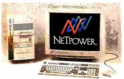
THE SYMETRA PENTIUM PRO dual-processor NT workstation is aimed at users seeking an alternative to RISC-based UNIX systems.
