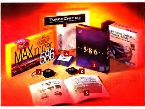
FIVE EASY PIECES: A CPU upgrade kit usually contains 1 a box, natch; 2 a processor; 3 a heat sink (it often comes attached to the processor); 4 a demo disk, with varying degrees of usefulness; and 5 an illustrated manual, written in plain, nontechnical English—if you're lucky.
