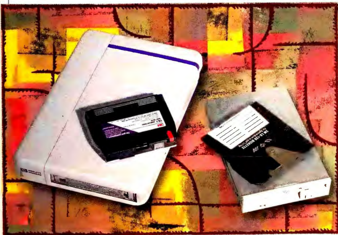
MAGNETIC CHARM: For self-employed users with older PCs, magnetic tape backup drives such as HP Colorado Memory Systems' T1000e, with its 800MB capacity (left), are cheap. Another solution: OR Technology's a:drive (right), which stores 120MB on one floppy.
