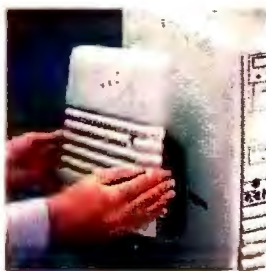
Removing the left-hand quick access panel provides easy access to expansion slots
