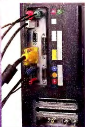
TOSHIBA USES color codes and icons to cut setup time to minutes. The bottom slot is occupied by a cable TV tuner and an FM radio card.
