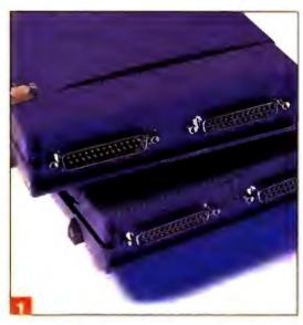
Identify the connectors. A parallel drive (top) has one 25-pin male connector for the cable to your PC and one 25-pin female connector for your printer cable. A SCSI drive has one connector for the PC cable and one for another SCSI device's cable.
