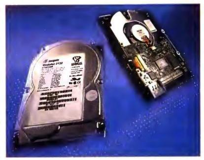
using bundled software: The GOOD COVER-UP: The Seagate Medalist 2132 (left) is fully shielded. Circuitry on most drives, such as the unit at right, is exposed.
