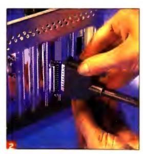
Hook up to a parallel port. Shut down your PC. Disconnect your printer cable if you have one. Connect your PC's parallel cable to the parallel drive's connector. If you've got a printer, connect its cable to the rear of the drive. Go to Step 5.
