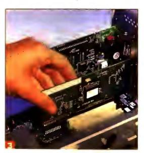
Hook up to a new SCSI adapter. If your PC has a SCSI port, skip to Step 4. If not, you'll need a SCSI add-in card. Shut down your PC, remove the cover, and follow the directions that come with the SCSI card. Connect the drive to the card. Go to Step 5.
