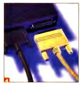
Hook up to an existing SCSI adapter. Shut down your PC. Connect the cable from the removable cartridge drive to your PC's external SCSI connector. Set the drive's SCSI ID; you may also need to set your adapter to recognize an external drive. Go to Step 5.
