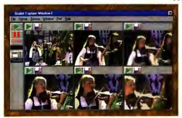
FIGURE 1: CAPTURE FRAMES FROM FULL-MOTION VIDEO with Alms Lab's Grabit, a parallel port device.
