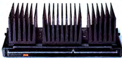
THE PENTIUM II resides in Intel's Single Edge Contact cartridge, attached to a huge heat sink; NEC's version is shown.
