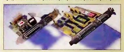
Install the card. Back up your data, turn off your PC, and then remove the PC's case. If you're replacing an old I/O card, take out any mouse or modem cables that are connected to It and remove the card.
