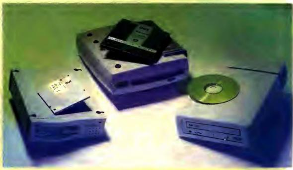
SERVE YOUR FILES ON A SILVER PLATTER-drives from left to right: Fujitsu DynaMO 640, Pinnacle Micro Apex 4.6GB Optical Hard Drive, and HP SureStore CD-Writer Plus Model 7110.
