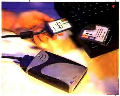
doesn't come with a spare DOCKET IN YOUR POCKET: Avatar's 250MB Shark drive is the SCSI connector, you'll most smallest drive here, and it draws its power off the computer.
