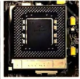
FIGURE 2: TO DETERMINE THE SOCKET your CPU is plugged into, read the label.
