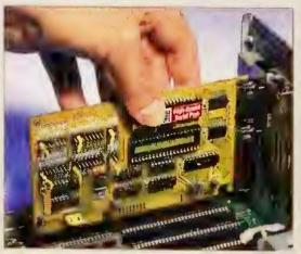
recent model, settings should be handled by Plug and Play. With older PCs (or Windows 3.x), you'll have to set up a jumperless card using the Included software.
