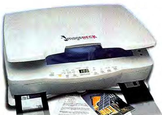
NO PC REQUIRED: Microtek's stand-alone ImageDeck scanner features built-in Zip and floppy drives for saving its scans.
