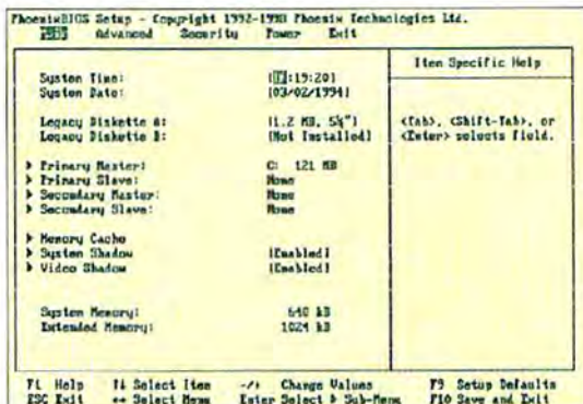
FIGURE 1: INSTALL YOUR hard disk in the CMOS setup program. Select the configuration that matches your system.
