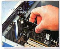
2 Set the SCSI ID number and terminate the drive. SCSI drives must be set for a unique ID number, which is set by jumpers (A) on the drive. If your SCSI removable-media drive is the only SCSI drive in your PC, the default ID (usually 4 or 5) is fine. If you have other
