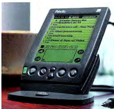
PALM LITE: The Palm IIIe looks like the IIIx but is about $70 cheaper and less expandable.
