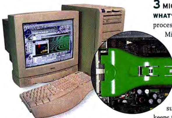
COOL COMPUTING: Special green ducting directs air over the Pentium III processor inside the OptiPlex GX1p 500. Keeping things cool can prevent some kinds of system crashes and lengthen a CPU's useful life span.
